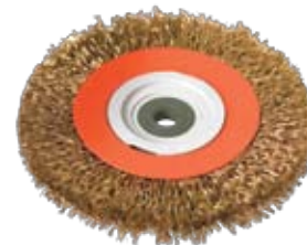
CCA - High Performance Wheel Traditional individual crimped wires (monofilaments) are substituted by crimped cables made of several wires each, resulting in 50% longer life than standard crimped wire.
