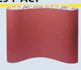
Abrasive belt with outstanding service life. Open coating, antistatic properties as well as ACT prevent premature clogging. The abrasive paper is particularly suitable for processing soft and high-resin woods
